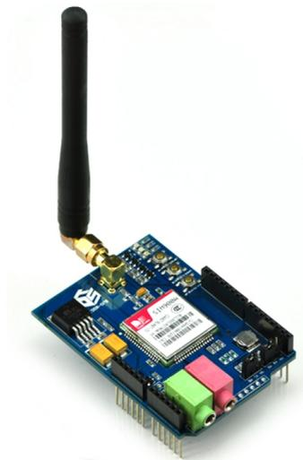
Figura 41 – Shield GSM SIM900.
